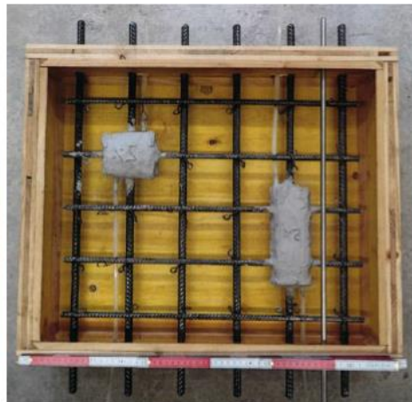
10x10cm Ø14mm (1 st layer), Ø10mm (2 nd layer). Cover = 18mm
