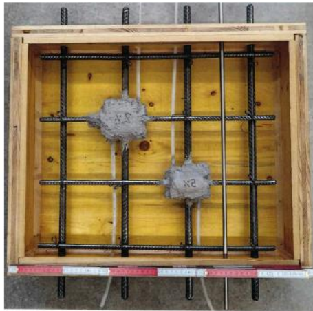
15x15cm Ø16mm (1 st layer), Ø12mm (2 nd layer). Cover = 18mm
