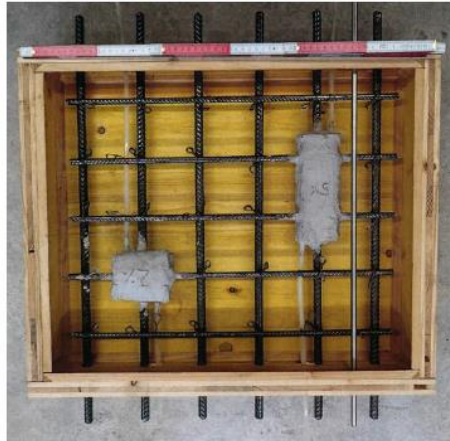
10x10cm \varnothing 10\text{mm} (1st layer), \varnothing 14\text{mm} (2nd layer). Cover = 54mm
