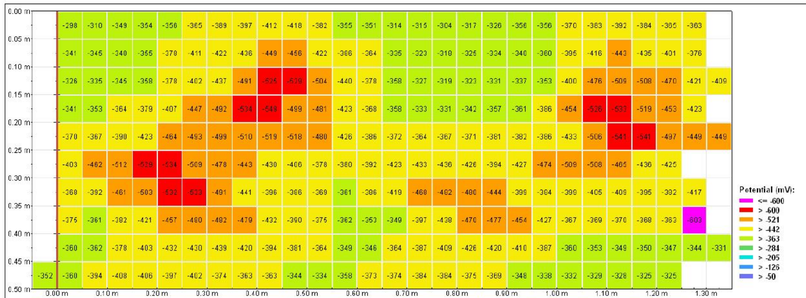
15x15cm \varnothing 12\text{mm} (1 st layer), \varnothing 16\text{mm} (2 nd layer). Cover = 54mm
